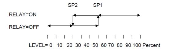
Eg The diagram above shows the relay operation against the level 0 to 10 for Parameter B0= RELAY START STATE (=OFF)
