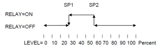
DELAY\_SETPOINT\_I and DELAY\_SETPOINT\_2 allow a delay for the relay to operate after the level exceeds the setpoint triggers LEVEL\_SETPOINT\_I and LEVEL\_SETPOINT\_2. These timers are reset when the level is between the LEVEL\_SETPOINT\_I and LEVEL\_SETPOINT\_2.
