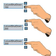
To edit a value press the ENTER key once, the display should now flash, now press the UP or DOWN key until the desired value is displayed.
