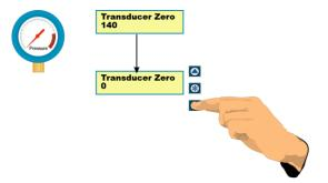
The level readings are averaged so the readings can lag behind the key presses. Always allow the system to stabilise prior to completing this procedure.
