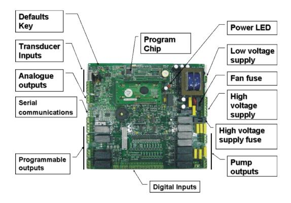
Detailed above are the locations for the components for the Hydrokos+ Printed Circuit Board (PCB)
