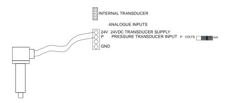
To use this input, note the wiring requirements on the PCB. A regulated 24VDC power supply is available on board for 2-wire configuration.
