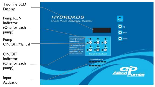
Each pump is controlled by an individual Auto / Off / Manual Switch.
